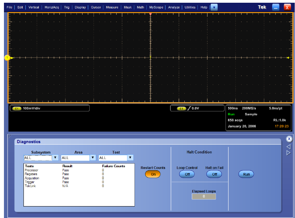
Figure 4-7: Diagnostics control panel
